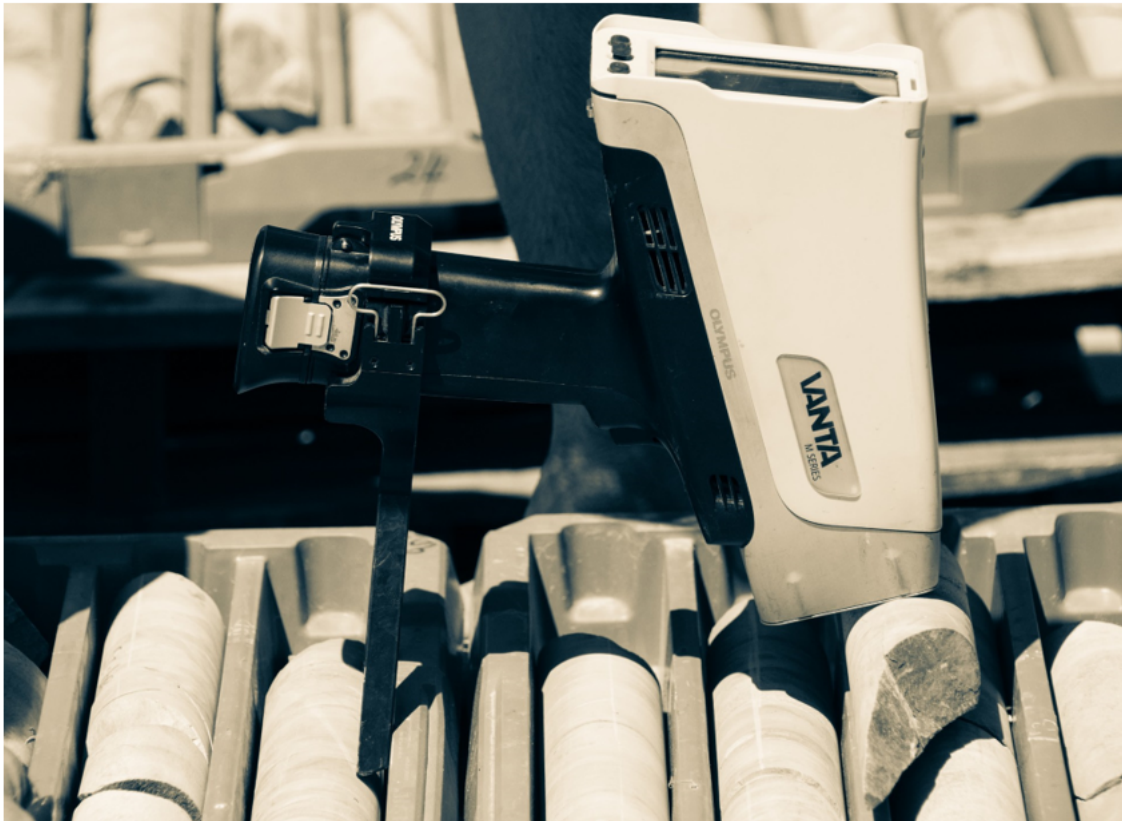
Portable X-ray fluorescence analysis (pXRF) is conducted by placing a hand-held instrument capable of in situ simultaneous multi-element analysis in contact with the sample to be analysed. Analytical results are immediately available for review by the operator.
