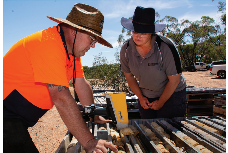
Figure 4: Geologists conducting XRF analysis of diamond drill core at the company’s core farm near Wedderburn.
